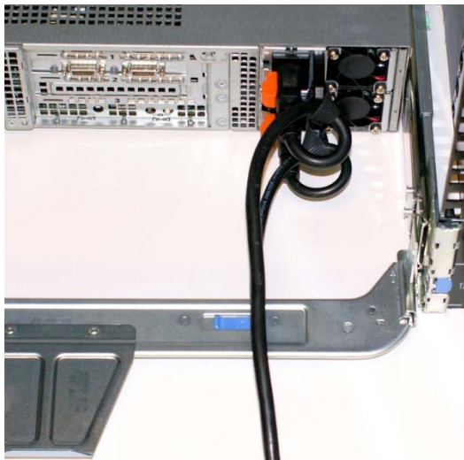
Figure 3: Routing Power Cables Through the Strain Reliefs
