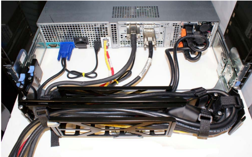
Figure 5: Left-Side Mounted CMA Installation
